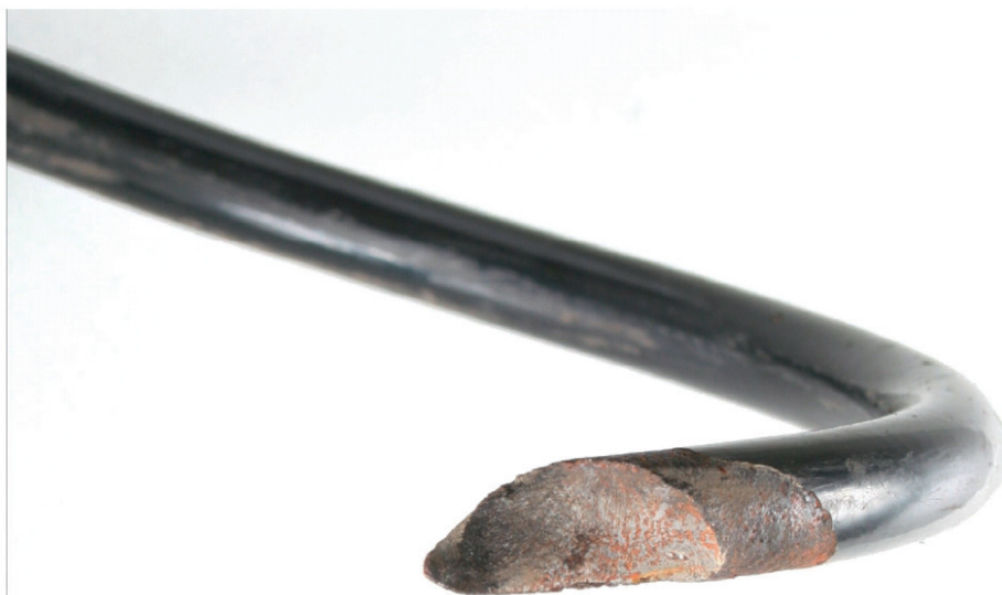
Typical, stress-corrosion fracture of a road spring
