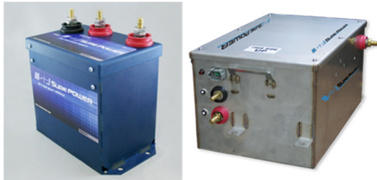
Figure 3. Heavy-duty supercapacitors feature two positive terminals, one for the engine starter and one for the battery. This prevents the battery from the constant wear and tear from typical engine start discharges.
